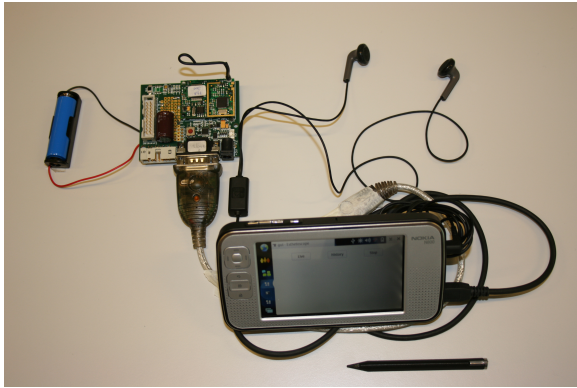
Figure 6. Sensor-Tune prototype: A linux-based PDA connected through a serial port to a wireless sensor
